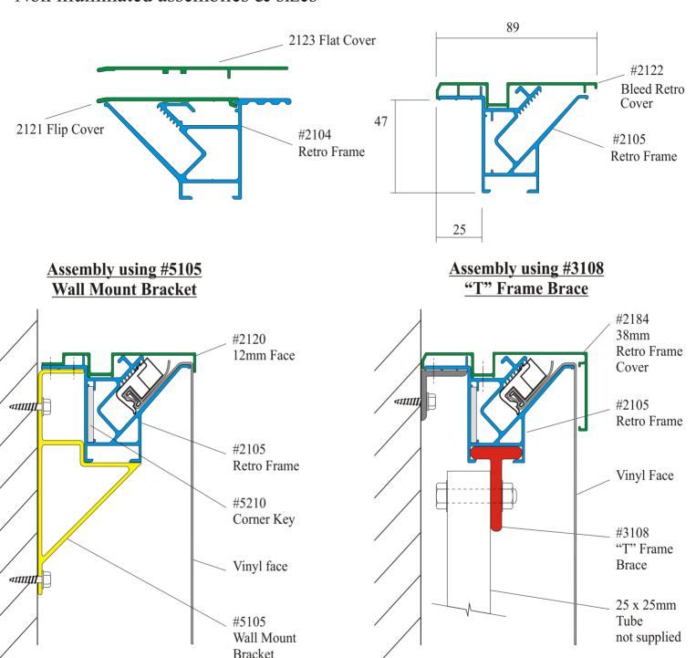
Place the #5105 Wall Mount Bracket or the #3108 "T" Frame Brace on maximum 1000mm centres. Where frames join, a #5105 Wall Mount Bracket should be placed each side of the frame joint. (For signs of more than 4000mm in height, reduce spacing to 600mm)
